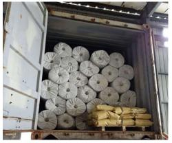
Infraclay GCL Dam Liner is normally supplied rolled on 100mm I.D. corrugated HDPE cores 5m wide x 30m long (area 150m2). Rolls 5.8m x 35m are also available. The liner can be cut to length or shape, as required. Each roll is packed in a strong waterproof liner to prevent water absorption and loss of rigidity during transportation. Lifting slings can be fitted on request. Bentonite granules and powder is also available.
