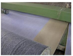
GCLs have been used in environmental, civil and landfill liner applications for nearly 30 years. They have an unmatched sealing capability and are cheaper to install than compacted clay soil. Rolled out like a carpet and hydrated with water, Infraclay GCL becomes a durable impermeable liner. Its self-healing around holes or punctures means there is less chance of leaks due to installation damage.
